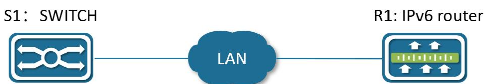
Typical network diagram of SLAAC address allocation
